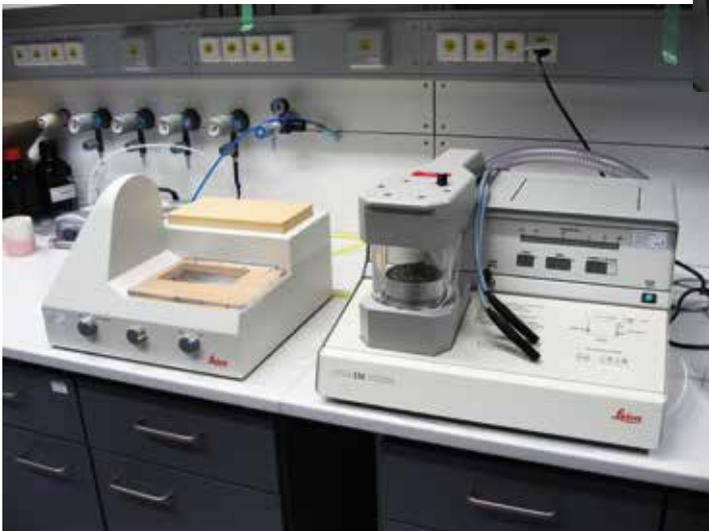
Fig. 3: Docking station and Carbon sputtering coater.
