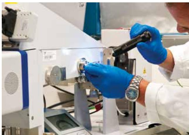
Fig. 1: Loading a sample into the SAXS instrument.
