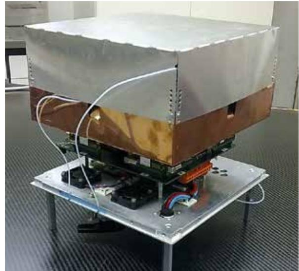
Fig. 1: A bare CASCADE system in 20x20 cm<sup>2</sup> with active detection volume (aluminum cover) and readout electronics (below)
