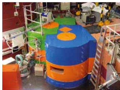
Fig. 2: The new biological shielding at SR 9a (blue-orange) between instruments HEiDi (green-orange) and RESI (rose-red).
