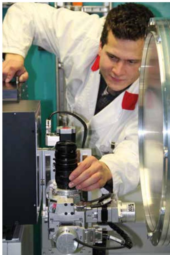
Fig. 3: Philipp Schmakat is placing a sample on the new stage for small samples in the first experimental chamber.
