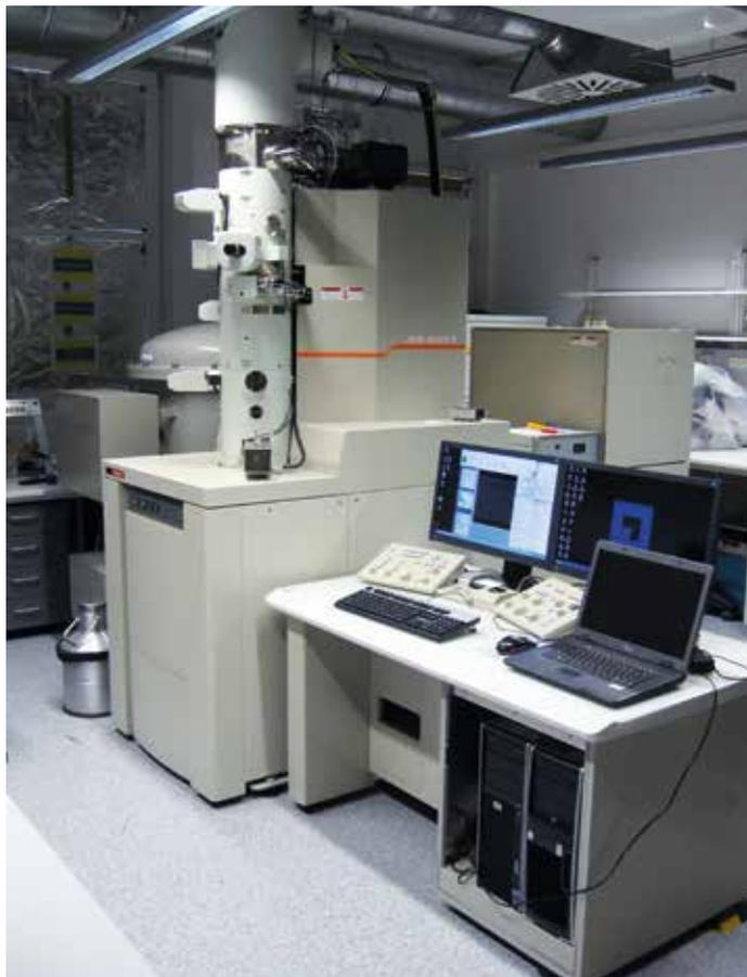
Fig. 1: JEM-FS2200 Transmission electron microscope at JCNS@FRM II.
